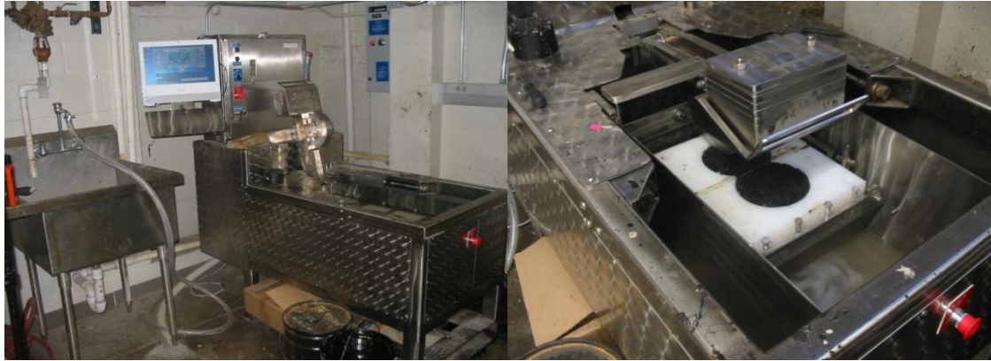
FIGURE 4: Hamburg Wheel Tracking Device and specimens ready for testing.
